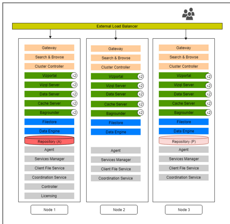
Figure 5 Example of a basic 3-node HA deployment.
