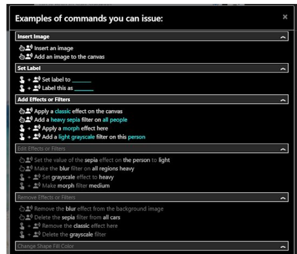
Figure 2: A list of commands suggested in the Exhaustive Interface. In this case, commands for editing and removing filters are faded out because the user has not applied any filters yet.
